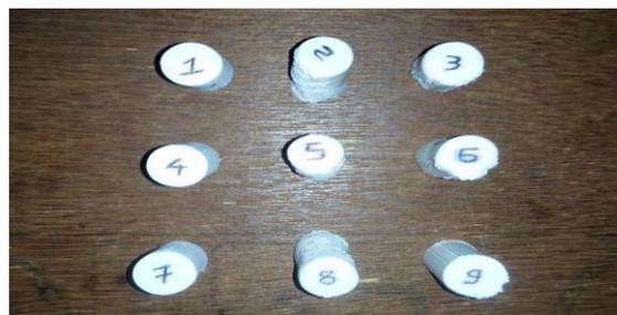
Fig.2 Compressive specimen after test
